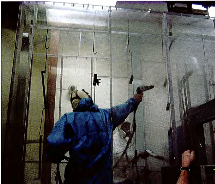
Powder coatings that provide maximum protection from the hot Nevada sun are applied in a temperature-controlled environmental room.
