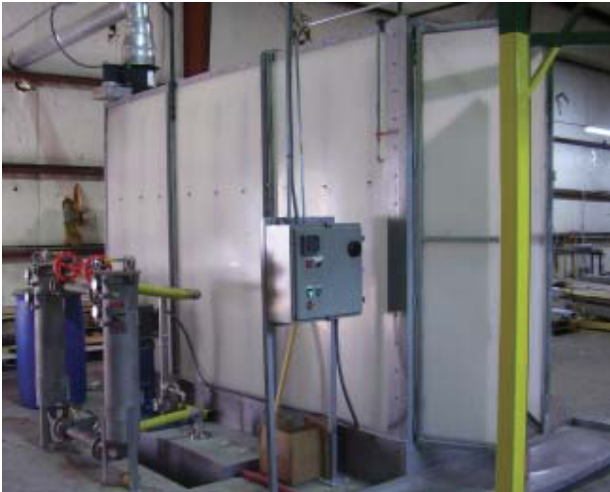
Figure 3: Small, efficient batch spray washer: parts are pretreated and dripped off on manual or automatic cycle.
